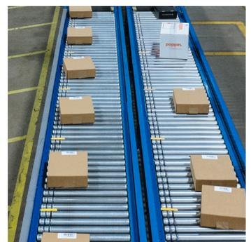
To keep product running smoothly on the solution, eliminate any catch points, and focus on guarding. Irregular products are prone to catching on these points or getting caught in gaps. Take even the smallest openings off of the table to ensure product doesn't snag or catch during transport.
