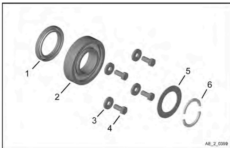
Figure 5.8: 100% replacement parts after propeller strike
