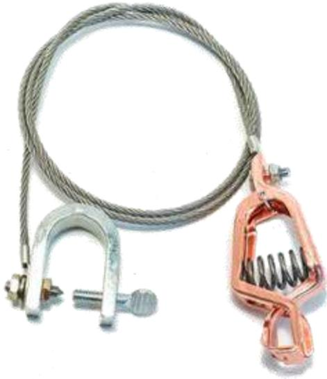
Items such as drums and tanks can have their conductivity affected by paints, coatings, or a buildup of product. These coatings can be thick enough to keep electrostatic charges from dispersing altogether. The solution is to use a grounding assembly with clamps that can pierce paint for a good metal-on-metal connection.
