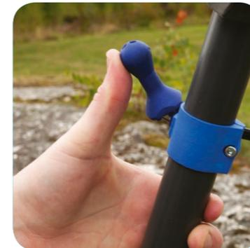
Move the handle up to temporarily release the compass.
