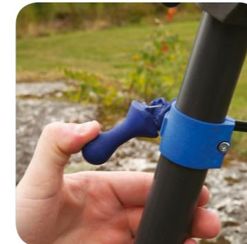
Move the handle down to temporarily release the reverse brake.
