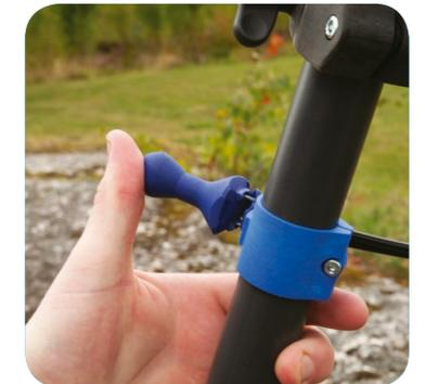
Move the handle sideways to temporarily release both the reverse brake and the compass
