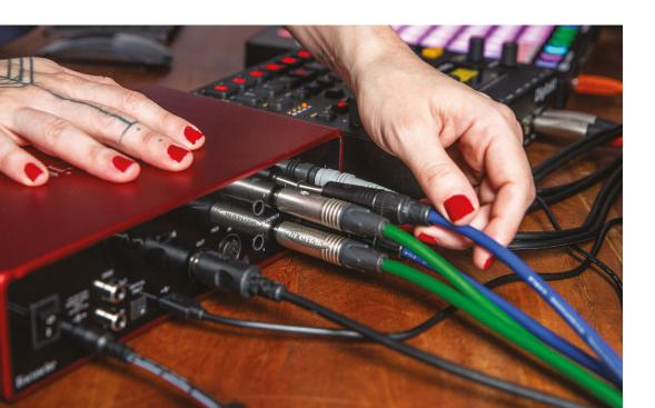
An 'unbalanced' connection only relies on two points of electrical contact. Accordingly, unbalanced cable only has two wires: a ground and a signal. In an unbalanced connection, the ground wire performs two duties: it shields the signal wire from interference, and also carries part of the audio signal. Unbalanced connections are prone to picking up interference, and should be kept short to avoid noise in the signal.
