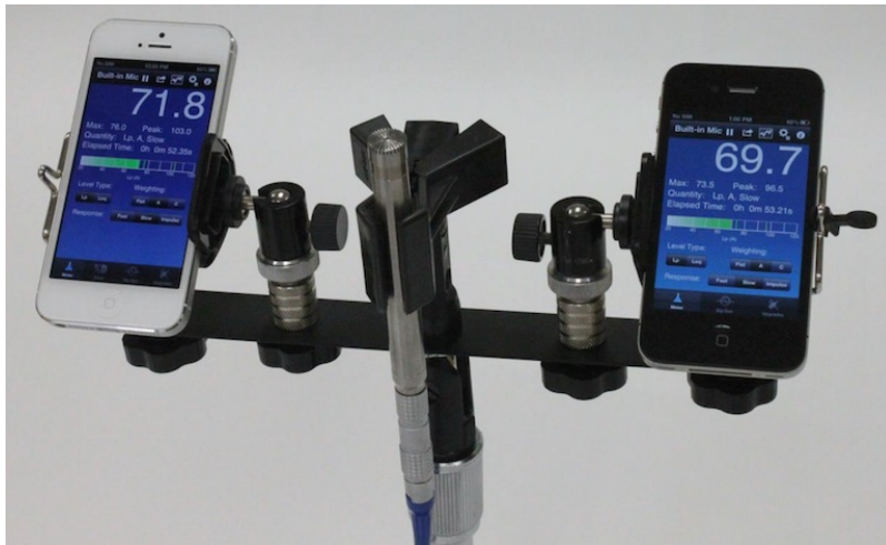
Figure 3. A suggested procedure for measuring and comparing smart phone sound level meter (SLM) apps. The SoundMeter app on the iPhone 5 (left) and iPhone 4S (right) compared to ½" Larson-Davis 2559 random incidence type 1 microphone (center). From Kardous and Shaw, 2014). The smartphones were attached to a stand in the middle of the reverberant sound chamber at a height of 4 feet, and about 6 inches from the reference microphone.
