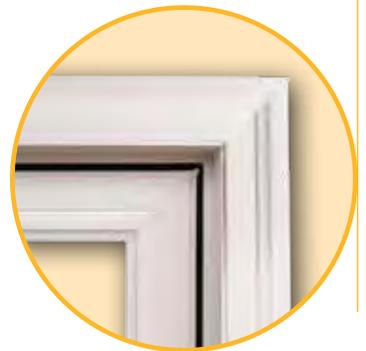
2" exterior brickmould profile provides a traditional style to an existing wood brickmould application. The profile overlaps the frame and has a "cutback" or extends 1-1/2" more than the frame.
