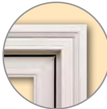
2-1/4" contoured brickmould application provides a modern style to an existing wood brickmould. The profile overlaps the frame and has a 2" cutback.
