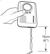
Turn the detector on its side so that the vents on the right hand side of the detector are pointing downwards. Hold the burning incense stick 15cm (6 inches) below the detector, so that the smoke enters the vents on the side of the detector. An increase in the localised carbon monoxide level within the sensor to more than 50ppm will cause the sounder to sound for one cycle of four loud beeps and the Fault LED to illuminate amber for a short time. This is the end of the test.
