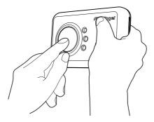
Cover the sounder vents with one hand. Press and hold the Test/Reset button down with your thumb/finger until the Fault LED illuminates amber and the sounder sounds for a second time (this should happen after around 5 seconds). Release the Test/Reset button. Upon releasing the Test/Reset button the Fault LED will flash amber once every second. This indicates that the sampling rate of the detector has increased and can be tested using a known source of CO.
