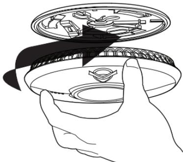
Once the smoke alarm has been fitted onto the base plate correctly, the internal power pack will activate. The red LED on the front of the alarm should now flash once every 40 seconds to show that it is active.
