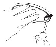
**3.** Fit Your FireAngel<sup>®</sup> Smoke Alarm Hold the alarm up to the base plate and push and rotate the alarm clockwise into position as shown. Make sure that the unit is securely fitted.
