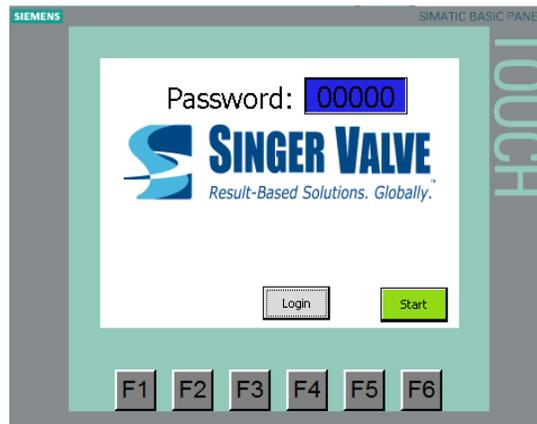
Touch the START button to complete the login procedure and move to Main System Window
