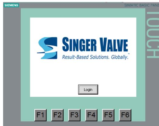
Touch the LOGIN button to enable the PASSWORD input box.
