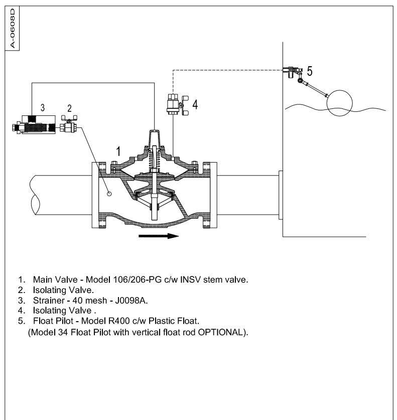
Pilot Operated Modulating Float Valve. ( 2 1/2" to 24" 106 / 4" to 36" 206). ---- connected in field
