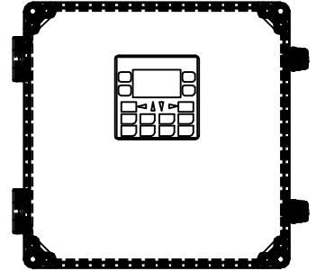
SCREEN AND KEYPAD INSTALLED ON AN INTERNAL DOOR
