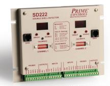
The SD222 System offers double end detection for ends entering a conversion press, on a curler or traveling on the line throughout the plant. The SD222 is a dual-channel system, providing protection for two lanes, when paired with four non-contacting sensors. The SD122 is a single channel/one lane version that is also available.
