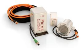
Prime Controls offers complete end light leak detection for high-speed EOE conversion presses with its Light Leak Detection Series. The detection series is comprised of the LH200 Light Head Sensor and SL100 LED Strobe Lamp. The system will detect holes through metal can ends on a conversion press with leak diameters 5 microns and below — outperforming industry requirements, and at rates over 1,100 ends per minute.
