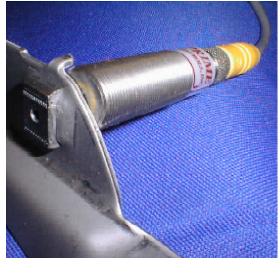
Detects ferrous metal through metal in the foreground
