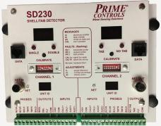
Each channel has three solid-state outputs. The infeed (shell) outputs energize for single end, double end and fault conditions. The discharge tab outputs energize for tab presence, no tab presence and fault conditions. Fault outputs indicate failure of internal components or an external probe failure.
