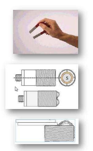
Magnetic thickness detection measures the shunting of a magnetic field across the north and south of a probe face. The magnetic shunt is proportional to the ferrous metal thickness. This method will not work on nonferrous metal.
