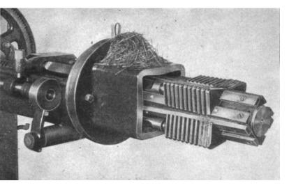
Broaching is a machining process using a cutting tool with teeth that increase in size from front to back. In many cases, an entire surface (or multiple surfaces) can be finished in a single pass with broaching. The technique is most often employed to finish holes, splines and flat surfaces.
