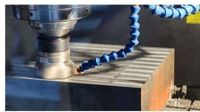
Above: CNC face milling Opposite: CNC slot milling
