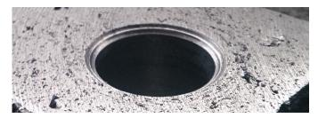
Above: a stepped hole formed by drilling Opposite: CNC drilling with liquid coolant
