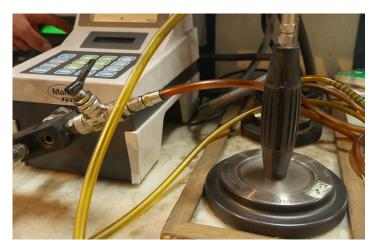
Air gages use pressurized air to measure the dimensions of an object. They were first introduced in the 1940s, and have undergone improvements to become one of the most trusted precision measuring tools in machine shops. Air gages function by shooting air out of a specifically calibrated nozzle, and recording the rate at which the air returns to multiple sensing nozzles. Thus, they are able to read the air flow between the measuring tool and the object being measured.
