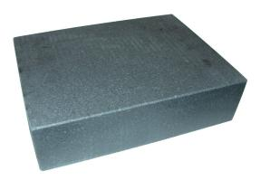
A surface plate is a flat surface used as a reference point for vertical (Y-axis) measurements. They're only useful if they're properly calibrated and maintain their shape impeccably. Because of its smooth surface and low level of expansion and contraction with temperature changes, granite is often the material of choice for surface plates.
