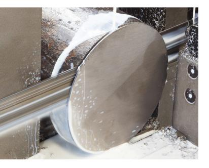
Sawing is one of the oldest cutting techniques in use today, and innovations have allowed the process to keep up with advances in material, tolerances and product complexity. By definition, sawing is cutting a narrow slit in a workpiece by moving a toothed or abrasive cutting tool against the surface. Sawing is often used to remove large sections of material without particular concern for tolerances, but modern CNC sawing machines can be used for finishing work as well.
