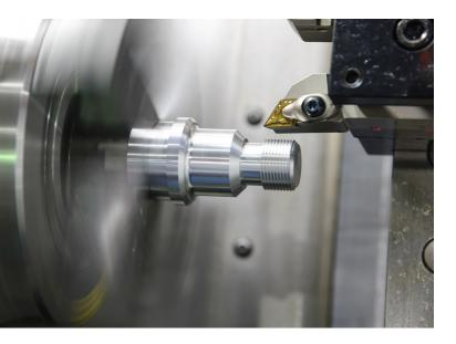
**Turning** has been practiced by machinists for centuries on many different materials. Originally, turning acted on wood to create complex, cylindrical designs for use in tools, handles and furniture. Today, turning is a vital part of the metal manufacturing process, and a major technique used by precision CNC machine shops around the world.
