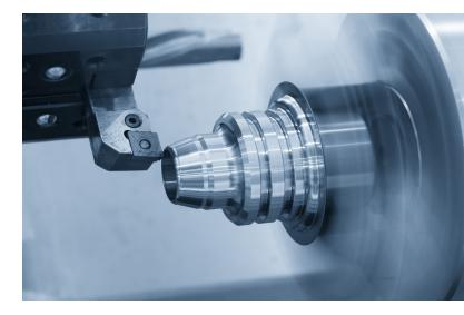
Above and opposite: turning processes on a CNC lathe
