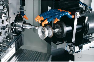
Above: a CNC grinding machine finishing tooltips
