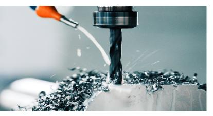
**Drilling** is one of the most common techniques used in manufacturing to create holes. In contrast to other hole-making methods like boring, reaming and tapping, drilling is most often used to create holes in unbroken surfaces. In precision CNC machining, drilling can range in scope from simple, rough hole drilling to complex, multi-feature hole drilling.
