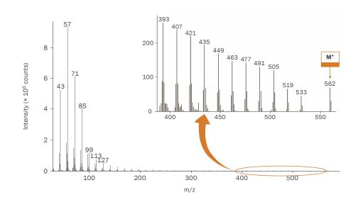
**Unlike other TOF mass spectrometers,** the spectral quality of BenchTOF results in excellent matches to 'classical' quadrupole spectra in commercial or custom libraries. In this example, the spectrum of tetracontane ( $C_{40}H_{82}$ ) shows preservation of the molecular ion.
