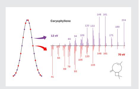
**One chromatographic peak, two complementary spectra. Rapid switching of ionisation energy enables reference-quality 70 eV and soft EI spectra** to be obtained simultaneously, without user intervention and in a single workflow.
