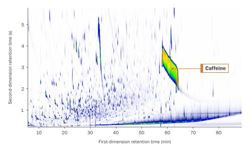
**Over 3000 components** were detected in this coffee extract using the high separation capacity of thermal modulation with cryofocusing, resulting in peak widths as narrow as 40 ms. Note the (predictably) high level of caffeine.
