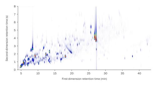
**Efficient and repeatable analysis** of volatiles in tobacco smoke was achieved using thermal desorption coupled with flow-modulated GC×GC–TOF MS. Optimisation of parameters revealed the complexity of this challenging whole-smoke sample, without the hassle and expense of liquid cryogen.
