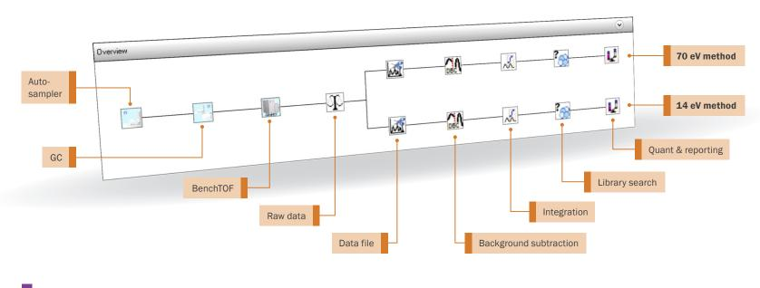
Tandem ionisation is fully integrated into the TOF-DS method workflow. with a simple graphical overview used to display each step from instrument control all the way through to reporting of results. Here we show the use of Tandem Ionisation at 70 and 14 eV, culminating in quantitative results for both ionisation energies.
