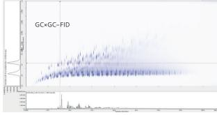
Fast and simple cross-validation, due to excellent retention time alignment between FID and TOF MS in this diesel sample analysed by parallel detection GC×GC.
