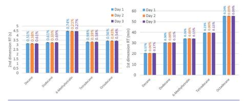
Excellent repeatability of retention times due to the use of a dedicated EPC for each column. The charts show retention time repeatability in the first and second dimensions for 24 injections over a 3-day period (n = 8 injections/day), with all RSD <1%.
