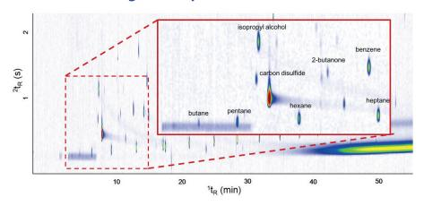
Insight provides efficient modulation of volatiles < C $_5$ . Here we show volatile compounds that are unable to be modulated by thermal devices.
