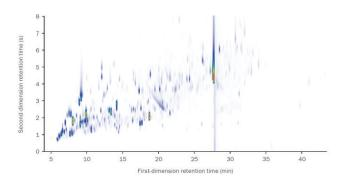
Here we show the analysis of whole smoke by thermal desorption-GC×GC-MS, with efficient modulation of volatiles. INSIGHT's flexible loop volume enables optimisation to minimise breakthrough of highloading components, such as nicotine.
