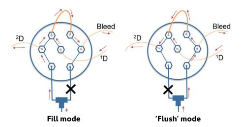
The valve-based Insight modulator uses differential flows to simply 'fill' and 'flush' a sample loop – meaning low running costs for routine GC×GC and none of the logistical issues associated with liquid cryogen.
