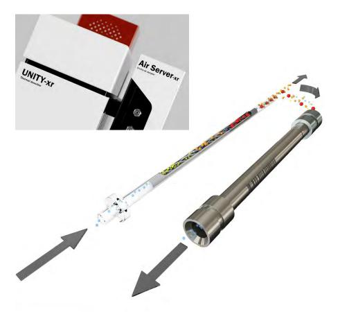
Focusing trap rapidly heated (up to 100° C/s) in a reverse flow of carrier gas ('backflush' operation), to transfer the analytes to the GC column.
