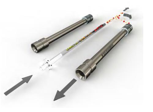
Focusing trap rapidly heated (up to 100° C/s) in a reverse flow of carrier gas ('backflush' operation), to transfer the analytes to the GC column.
