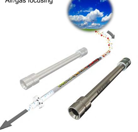
Samples are introduced directly onto the electrically-cooled, sorbent-packed focusing trap of the UNITY-xr thermal desorber, typically held between ambient and  $-30^{\circ}$  C.
