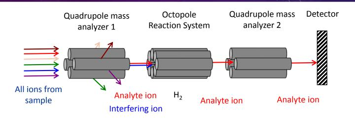
The ORS can be used with various gases (e.g., H<sub>2</sub>, He) to remove polyatomic interferences.
