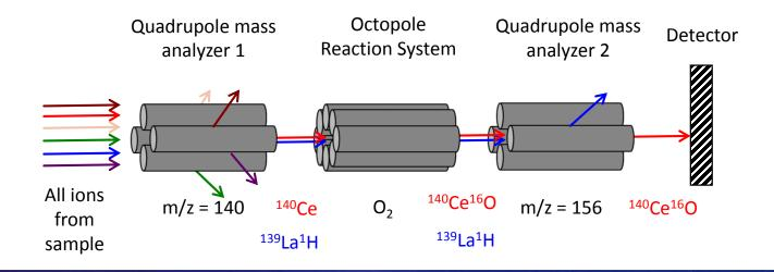
Or, the ORS can be used with gases (e.g., O<sub>2</sub>, NH<sub>3</sub>) to achieve a mass shift for the analyte thereby avoiding polyatomic interferences.
