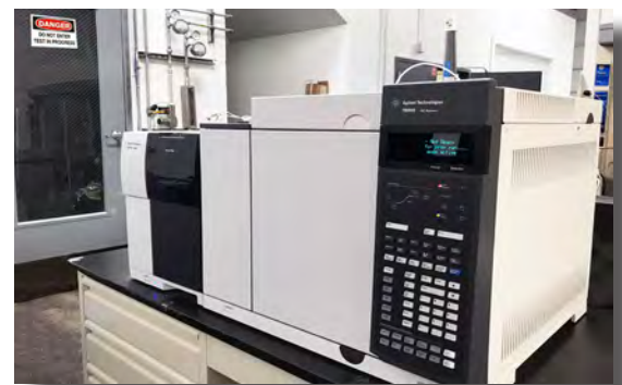
FAI uses an Agilent Mass Spectrometer and Gas Chromatograph in our flammability laboratory
