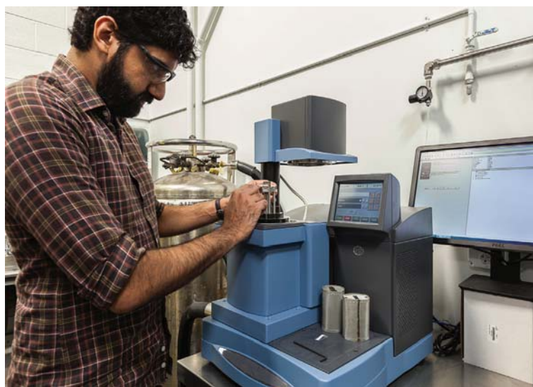
FAI utilizes the Q800 DMA manufactured by TA Instruments
