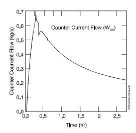
begins to decrease through the mechanisms discussed earlier. This figure also shows that aerosols are carried into the second room through counter current flow. The second plot shows that the counter current flow increases as the fire heats the first room, and decreases as the temperature difference between the two rooms decreases. The room cooling effect of the fire sprays leads to a reduction in the density differences and thus the counter current flow.
