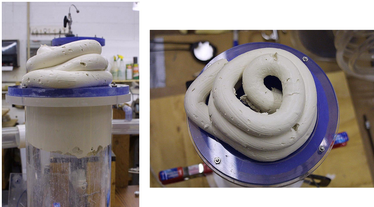
Figure 7. Extruded clay and residual clay left in test column after gas pull through.
