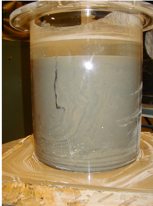
Figure 4. Settled Sludge After Transport. Only the lower four layers remain distinct; other layers have rotated or collapsed.
