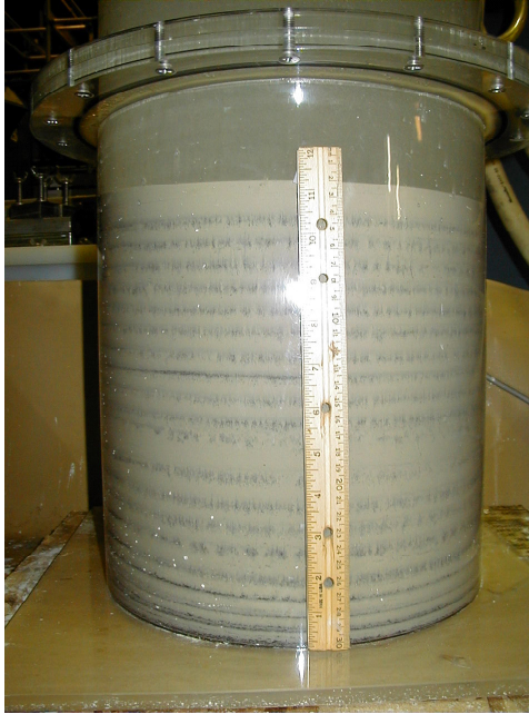
Figure 3. Settled Sludge Simulant, with 20 Distinct Layers Before Being Transported.
