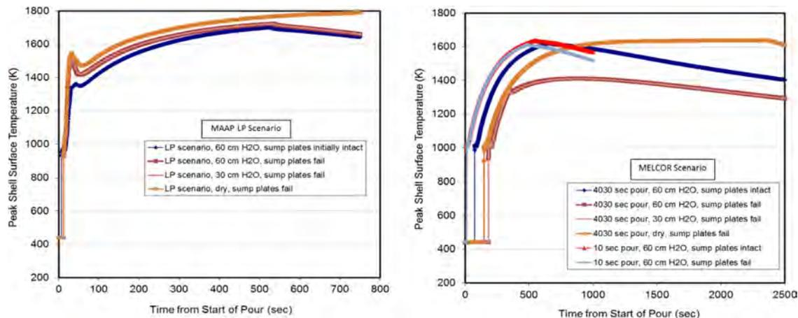
Fig. 8. MELTSPREAD predictions of liner heatup due to heat transfer from impinging melt for 1F1 based on a MAAP low pressure (LP) scenario (left) and MELCOR (right) melt pour conditions. (Courtesy ORNL, [56]).
