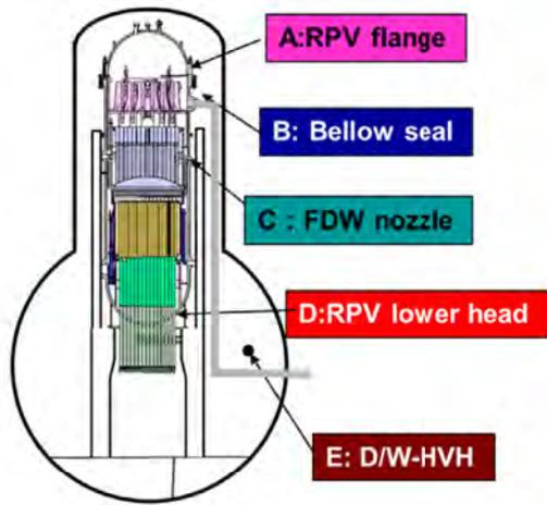
(a) Thermocouple position (RPV- reactor pressure vessel; FDW- Feedwater; D/W – Drywell; HVH -Heater Ventilating Handling)
