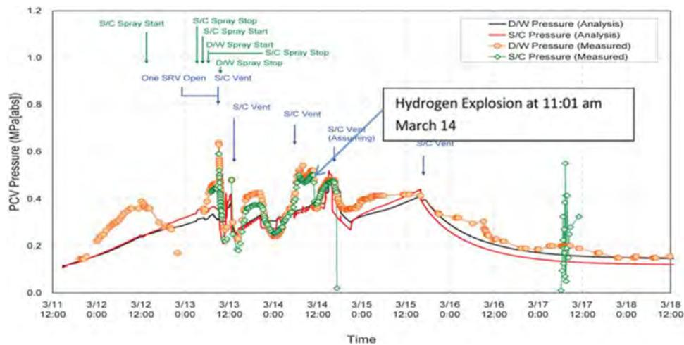
Fig. 15. 1F3 PCV pressure: the rapid drop coincides with 1F3 explosion time (Courtesy of TEPCO, [65]).
