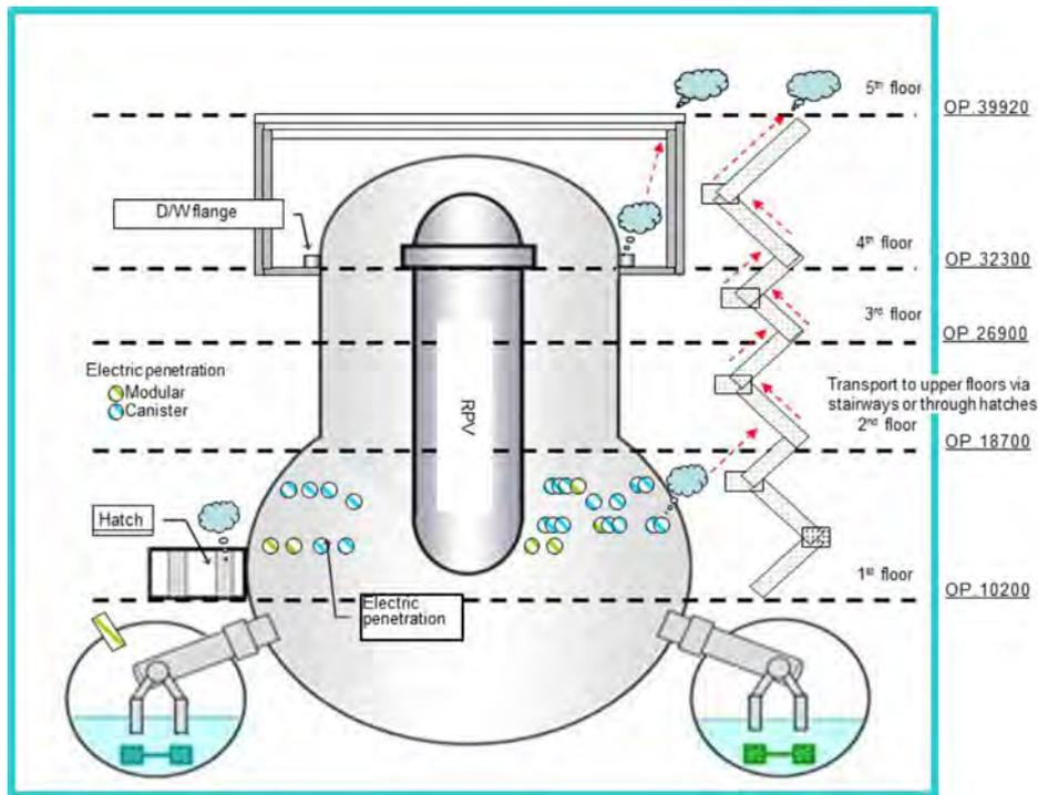
Fig. 10. Inferred hydrogen leakage paths. (Courtesy of TEPCO, [61]).
