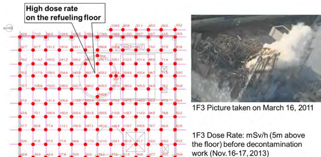
Fig. 3. 1F3 radiation survey (value in mSv/hr measured on November 16-17, 2013 at 5 m above the floor at points shown on grid) and photograph taken on March 16, 2011 (Courtesy of TEPCO [6, 8]).
