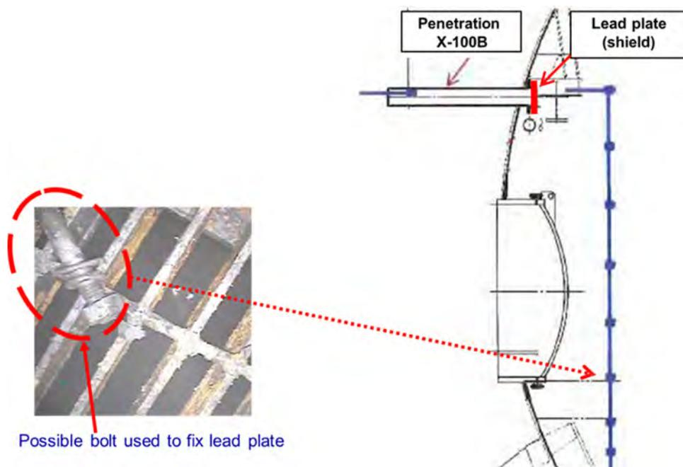
Fig. 1. Visual images within 1F1 X-100B penetration. (Courtesy of TEPCO [6]).
