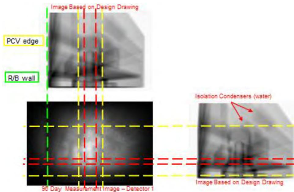
**Fig. 9.** Images of 1F1 obtained using muon tomography with scintillation detectors (the lower left image is measured; the other two images were calculated. Dashed lines are provided to show location of identified geometrical features). (Courtesy of TEPCO [10]).
