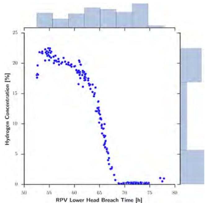
Fig. 16. MAAP 1F3 modeling uncertainty evaluation: refueling floor hydrogen build-up at time of 1F3 RB explosion. (Courtesy of EPRI [67]).
