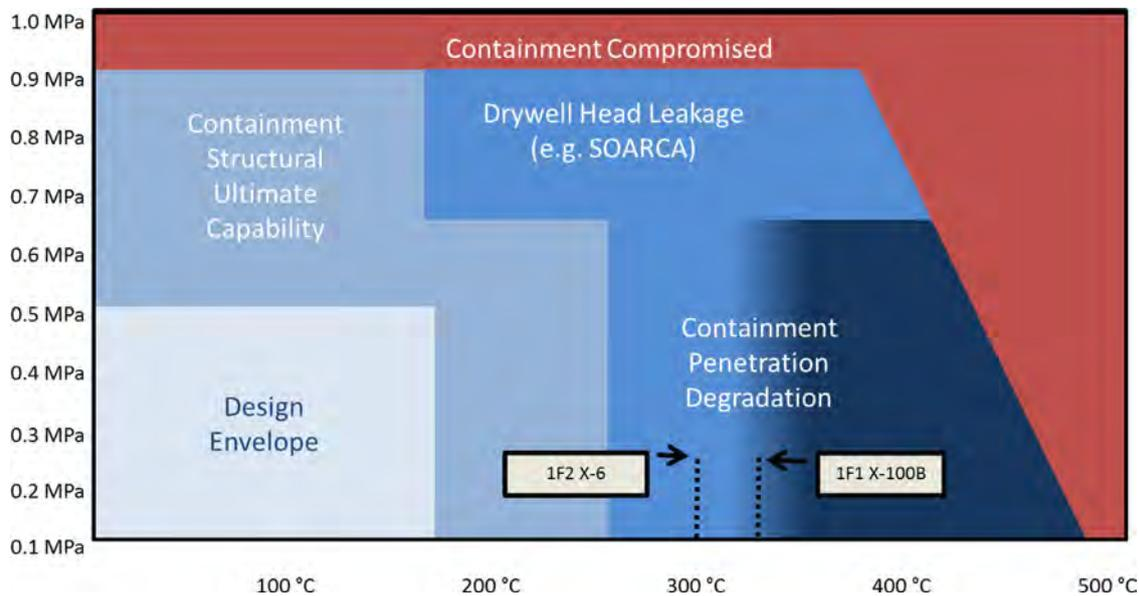
Fig. 4. Containment pressure/temperature curve with available 1F1 and 1F2 information. (Graphic courtesy of NEI [49] as modified by Jensen Hughes).
