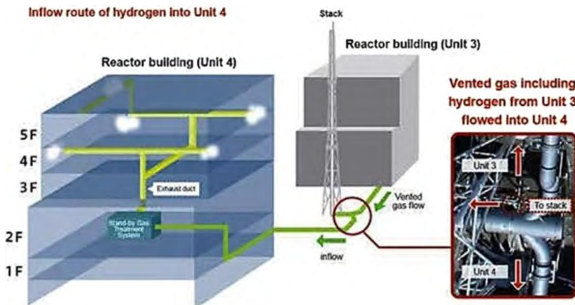
Fig. 11. Hydrogen transport path from 1F3 to 1F4. (Courtesy of TEPCO, [58]).
