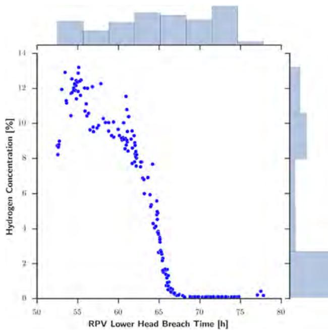
Fig. 17. MAAP 1F3 modeling uncertainty evaluation: fourth floor hydrogen build-up at time of 1F3 RB explosion (Courtesy of EPRI [67]).
