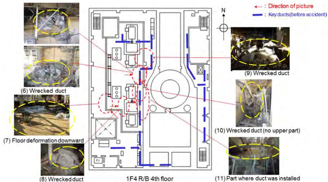
Fig. 13. Field investigation of the 1F4 4th floor (Courtesy of TEPCO, [61]).
