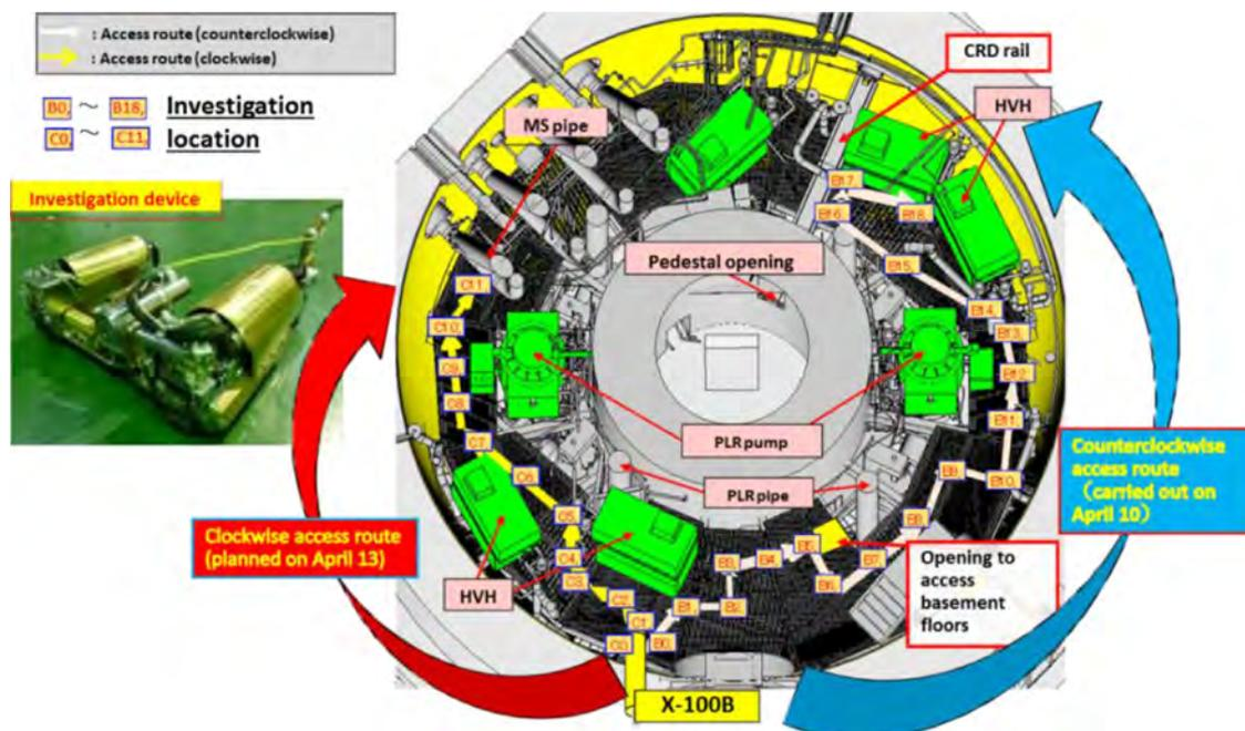
Fig. 6. Location of X-100B in 1F1 PCV and robotic examination paths completed on April 10, 2015. (Courtesy of TEPCO [55]).
