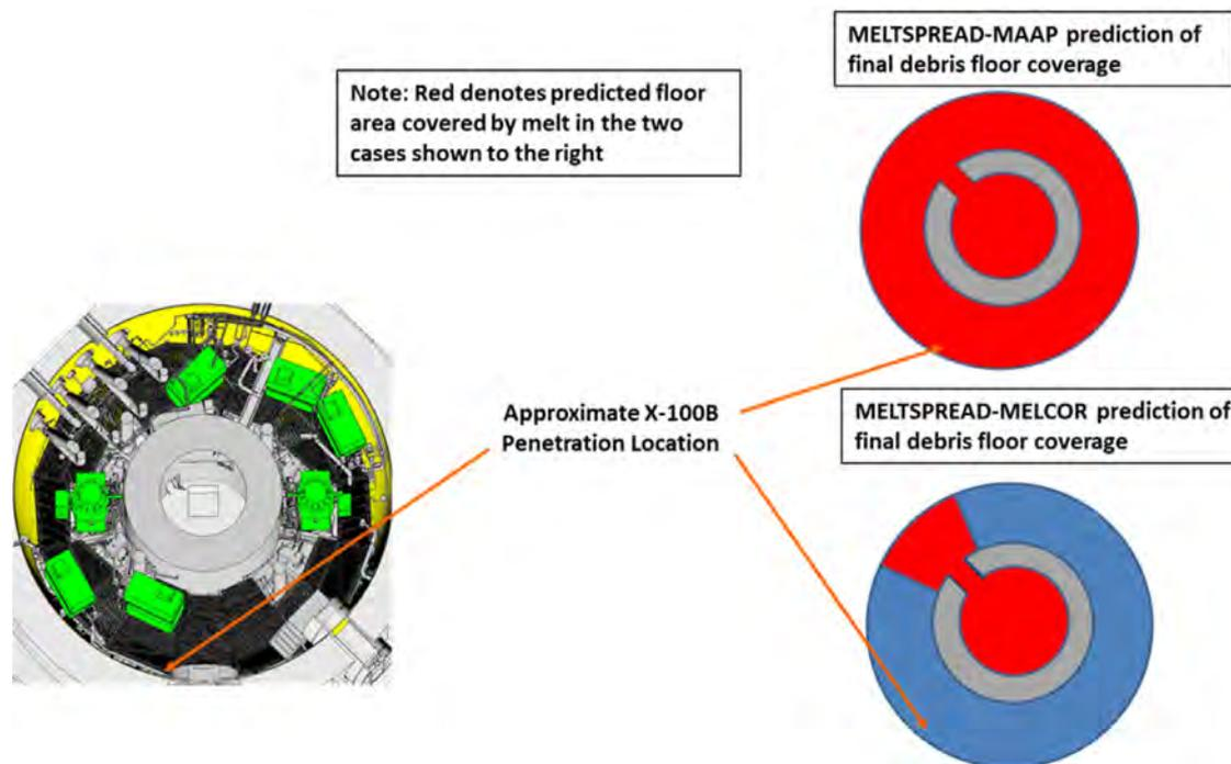
Fig. 7. Approximate Location of X-100B penetration relative to predictions of core debris spreading in 1F1. (Courtesy of TEPCO and ORNL [55, 56]).
