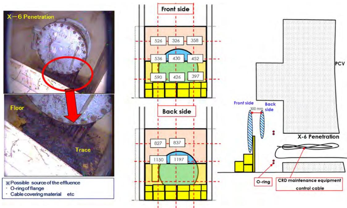
Fig. 2. Photographs and radiation surveys (in mSv/hr) near 1F2 X-6 penetration (values measured in 13 locations). (Courtesy of TEPCO [23,24]).
