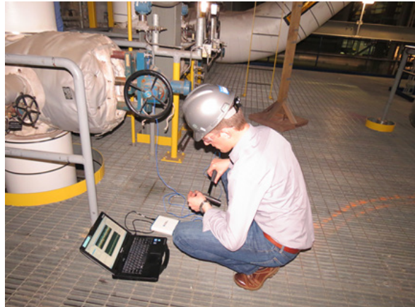
Figure 1 FAI Engineer Measuring Vibration Data on a Steam Valve Stem
