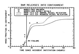
Figure 1 BWR Volatile Fission Product Release into Containment.
