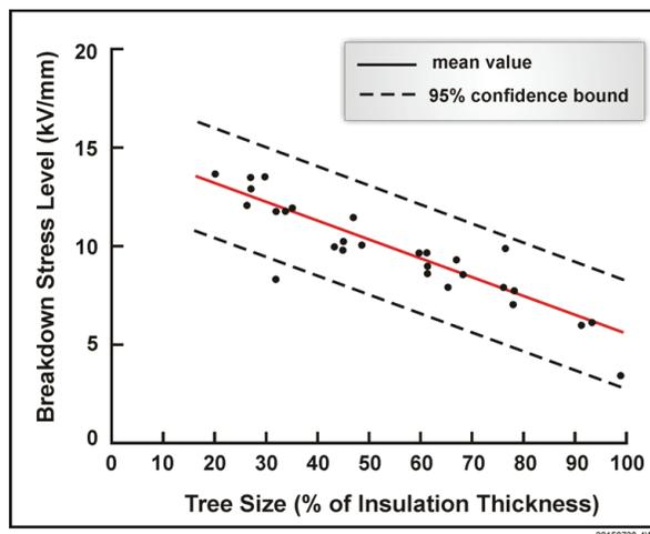
Figure 2: Breakdown stress vs. water tree thickness
