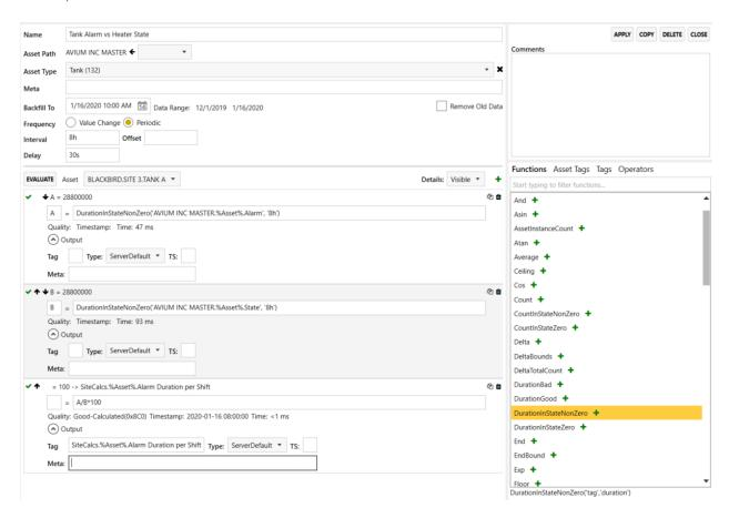
We have established A as the duration of time (in milliseconds) that the Alarm has been in nonzero form. B is the duration of time (in milliseconds) that the State has been in nonzero form. The final expression establishes a percentage by dividing the Alarm time by the State time and multiplying by 100
