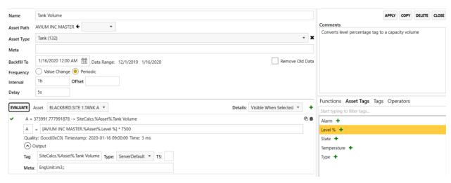
Here we are simply multiplying the Level % tag by 7500 to convert to a tank volume
