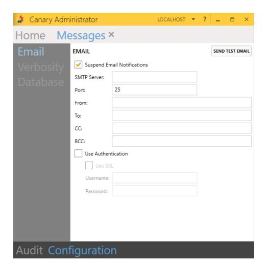
The "Configuration" tab allows setup of email notification and the message level for each source. To setup your email server, select "Email" at the left. The following will need completed.
