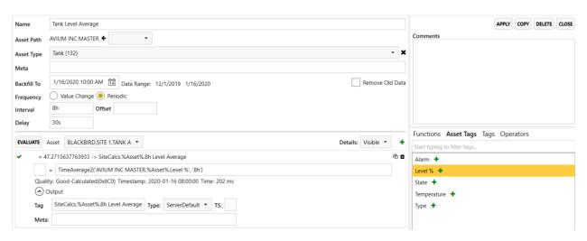
The TimeAverage2 aggregate has been used. The proper format is to remove the square brackets from around the asset tag and wrap it in single quotes. Then place a comma afterwards with a time interval to average within another set of single quotes.
