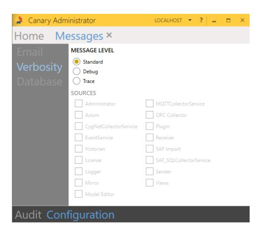
Additionally, at left is the "Verbostiy" menu. This may be configured to control/filter both the level of messages as well as their sources.
