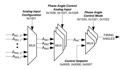
Figure 17 – Single Phase, Phase Angle Control Block Diagram
