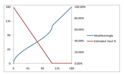
Figure 11 - Example Non-linear Conduction Angle vs. Output Voltage
