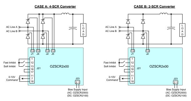
Figure 14 - Typical Single Phase H-Bridge Converter Applications
