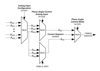
Figure 16 – Three Phase, Phase Angle Control Block Diagram
