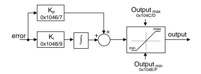
Figure 23 - Voltage PI Controller Block Diagram
