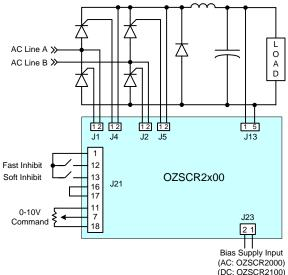
Figure 21 - Typical Single Phase Voltage Control Hardware Configuration
