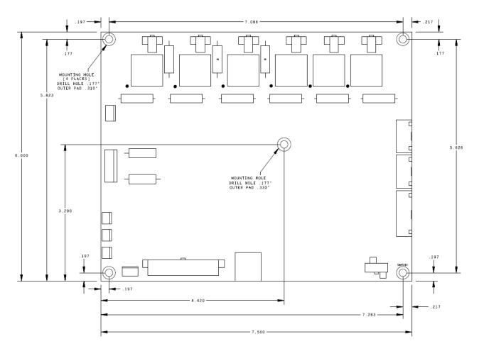
Figure 27 - OZSCR2x00 Mechanical Dimensions
