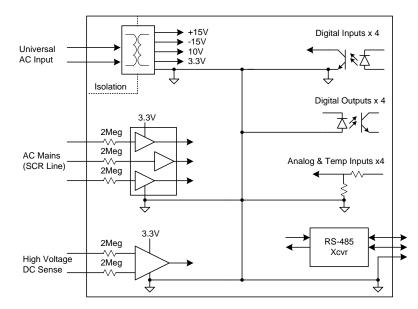
Figure 1 - OZSCR2000 Power and Grounding Block Diagram
