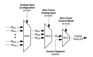
Figure 18 – Three Phase Zero Crossing Control Block Diagram
