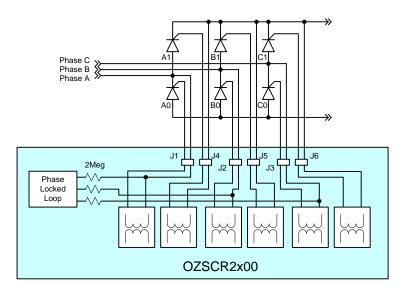
Figure 3 - Direct Line Synchronization Block Diagram
