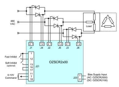
Figure 13 - Typical Phase Control 3-Phase Controller Application
