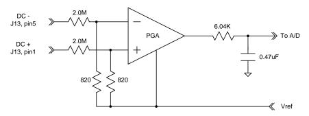
Figure 7 - J13 High Voltage Sense Interface Circuitry
