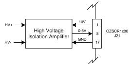
Figure 8 - Isolated High Voltage Sense Interface Circuitry
