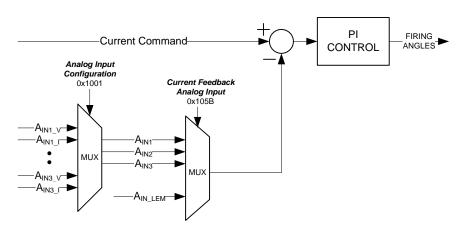
Figure 24 - Inner Current Loop Block Diagram
