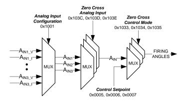
Figure 19 – Single Phase Zero Crossing Control Block Diagram
