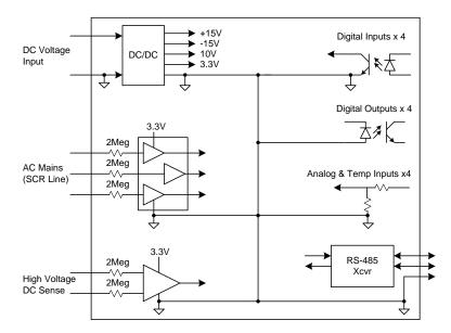
Figure 2 - OZSCR2100 Power and Grounding Block Diagram
