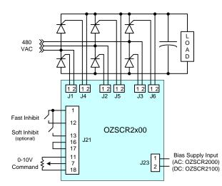
Figure 12 - Typical Phase Control 3-Phase Converter Application
