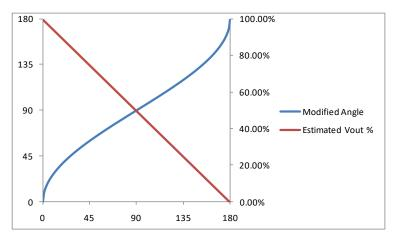
Figure 10 - Modified Conduction Angle vs. Output Voltage
