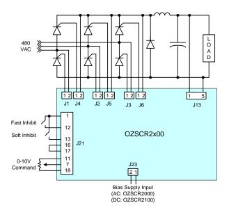
Figure 20 - Typical 3-Phase Voltage Control Hardware Configuration
