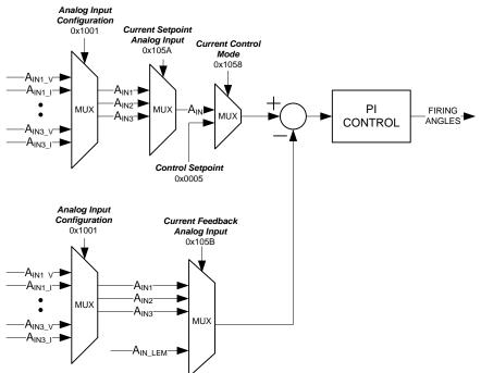
Figure 25 - DC Current Control Mode Block Diagram
