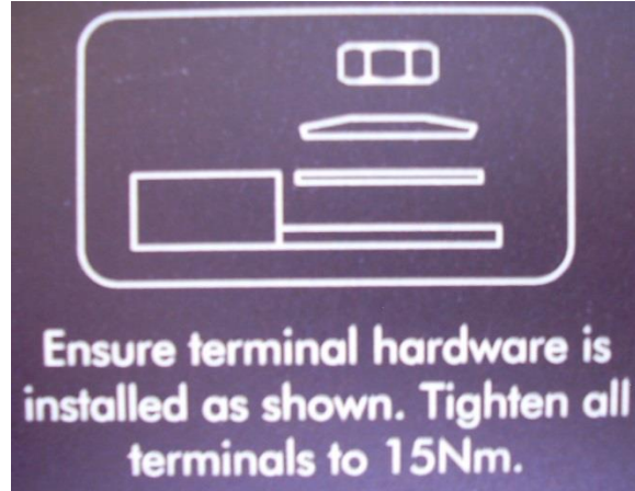
Figure 7: Power Terminal Hardware Stackup
