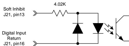
**Figure 6 - Soft Inhibit Electrical Interface**
