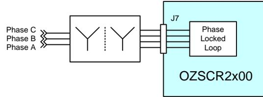
**Figure 4 - Low Voltage Line Synchronization Interface**
