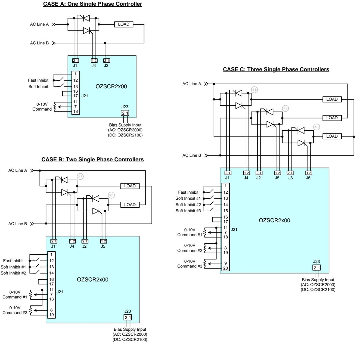
Figure 15 - Typical Single Phase Controller Applications
