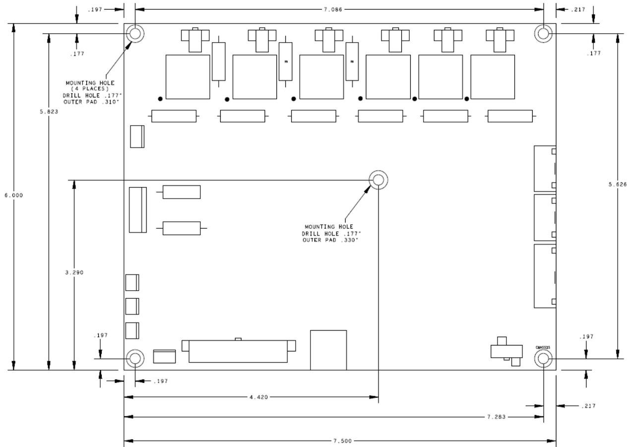
Figure 27 - OZSCR2x00 Mechanical Dimensions
