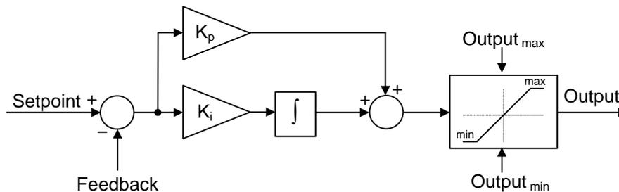
These parameters define the gain constants for the PI controller that is used to regulate the output current when operating in DC current control mode or in voltage control mode with the
