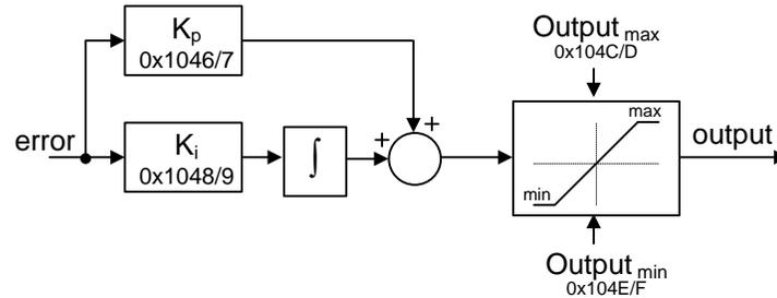
Figure 23 - Voltage PI Controller Block Diagram
