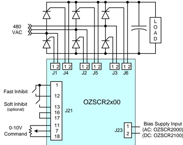
Figure 12 - Typical Phase Control 3-Phase Converter Application
