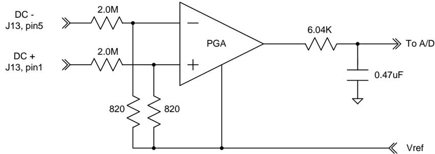
**Figure 7 - J13 High Voltage Sense Interface Circuitry**
