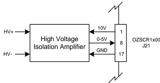
**Figure 8 - Isolated High Voltage Sense Interface Circuitry**
