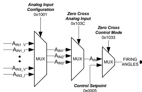
Figure 18 – Three Phase Zero Crossing Control Block Diagram
