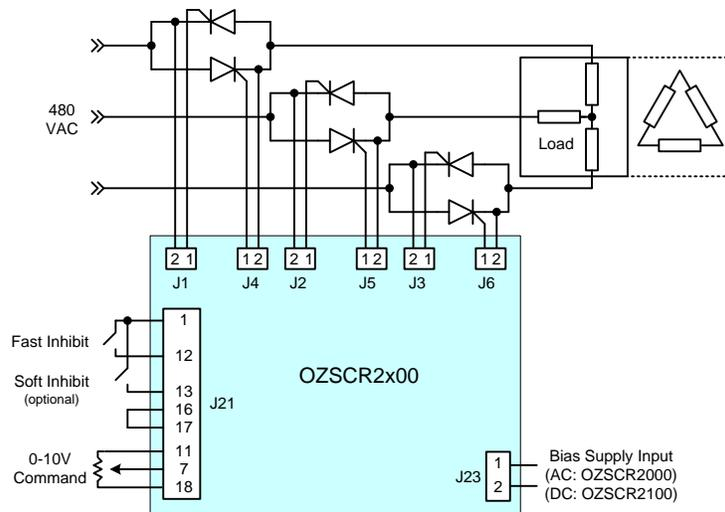
Figure 13 - Typical Phase Control 3-Phase Controller Application
