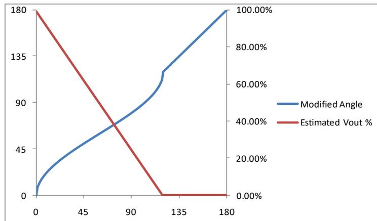
**Figure 11 - Example Non-linear Conduction Angle vs. Output Voltage**
