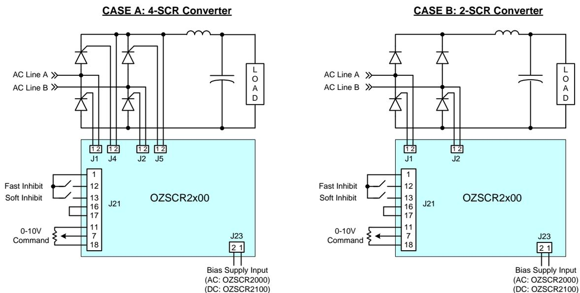
Figure 14 - Typical Single Phase H-Bridge Converter Applications
