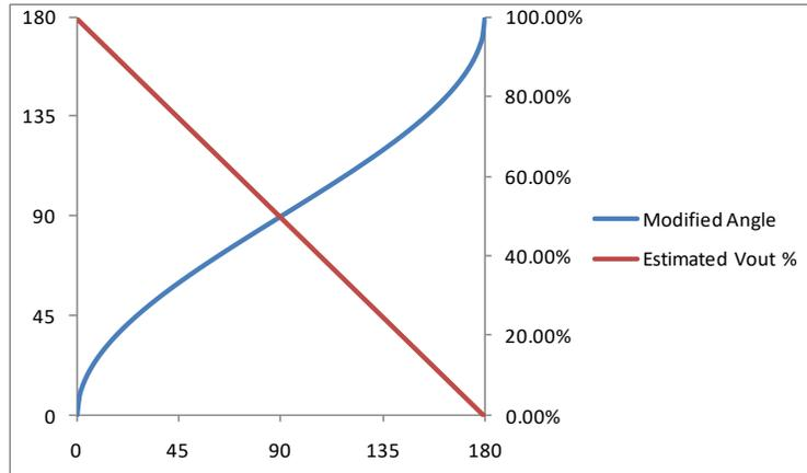
**Figure 10 - Modified Conduction Angle vs. Output Voltage**
