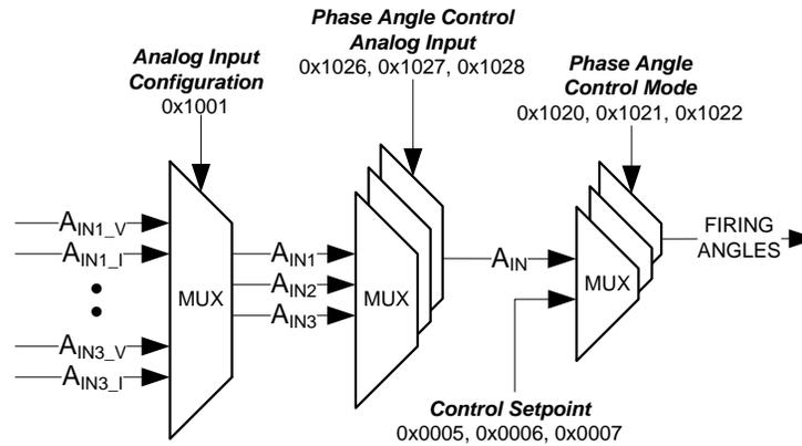
Figure 17 – Single Phase, Phase Angle Control Block Diagram
