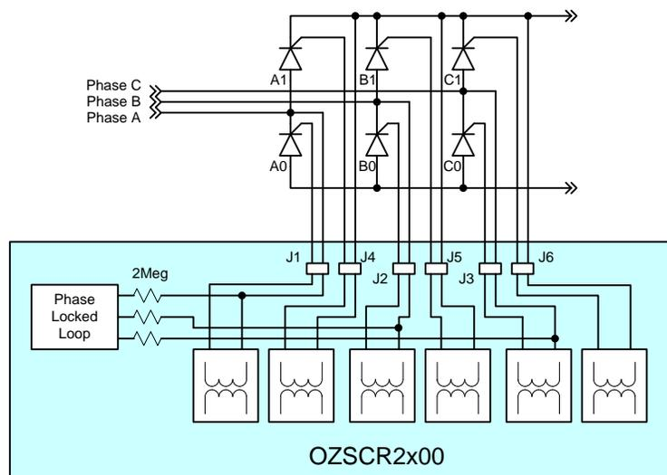
Figure 3 - Direct Line Synchronization Block Diagram
