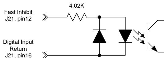
**Figure 5 - Fast Inhibit Electrical Interface**
