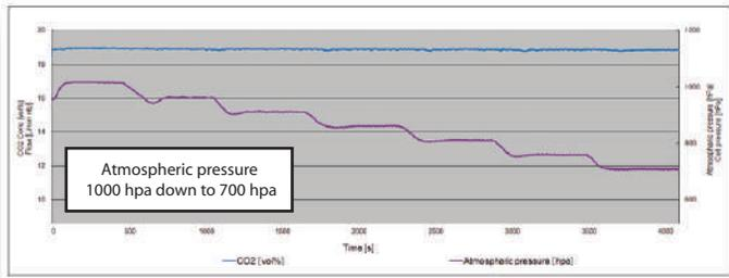
*Changes in atmospheric pressure do not affect the CO<sub>2</sub> level.*
