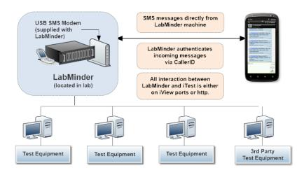
LabMinder typically sits inside the lab rather than on a company network, and is connected directly to an SMS modem.
