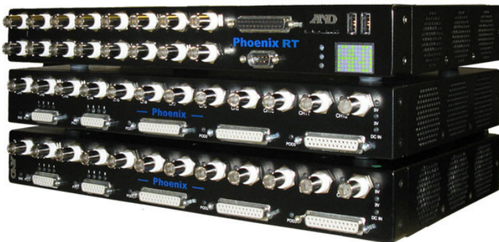
A 24-channel Phoenix system consisting of two Acquisition Modules (AM) and one Real-Time (RT) module.
