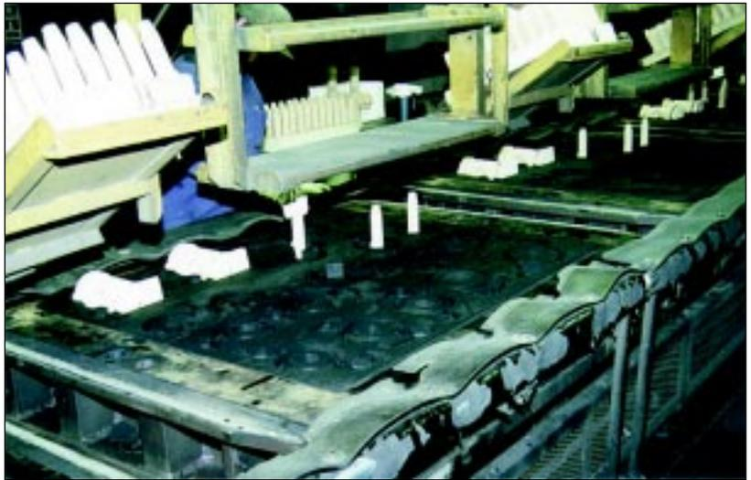
**A predominantly Western Bentonite sand binder can reduce the overall bond usage of a foundry by 10%. This will reduce overall molding costs for all types of molding lines and improve a foundry's bottom line.**
