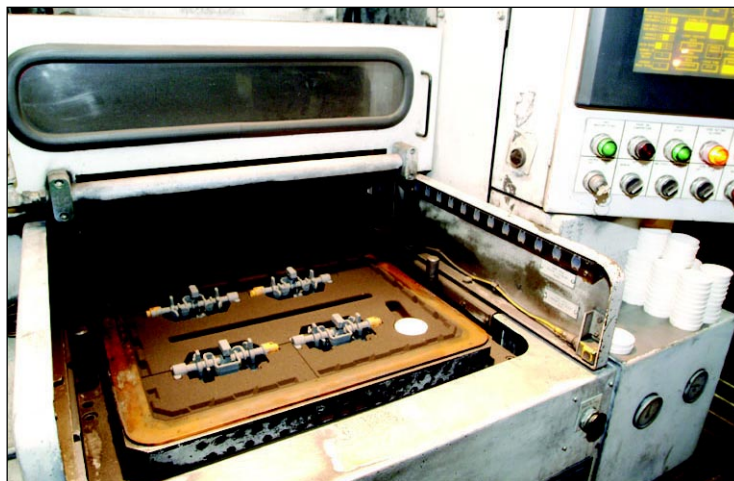
Through testing, a foundry that utilizes automatic matchplate molding (shown above) increased its level of Western Bentonite by 20% to achieve the desired sand characteristics.
