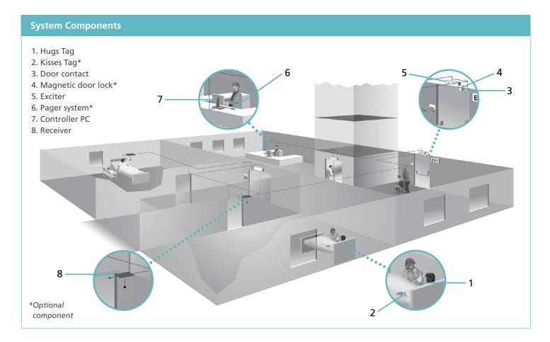
The Hugs tag contains a tiny radio transmitter. Once activated, the tag emits a special signal every 10 seconds indicating that it is present in the protected zone and is functioning.
