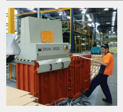
ORWAK MULTI is a range of top-loaded multi-chamber balers designed to facilitate sorting and compacting different types of material at source. The installation can easily be extended with additional chambers to grow in pace with your business and the multi-chamber solution can even form a mini-recycling station.
