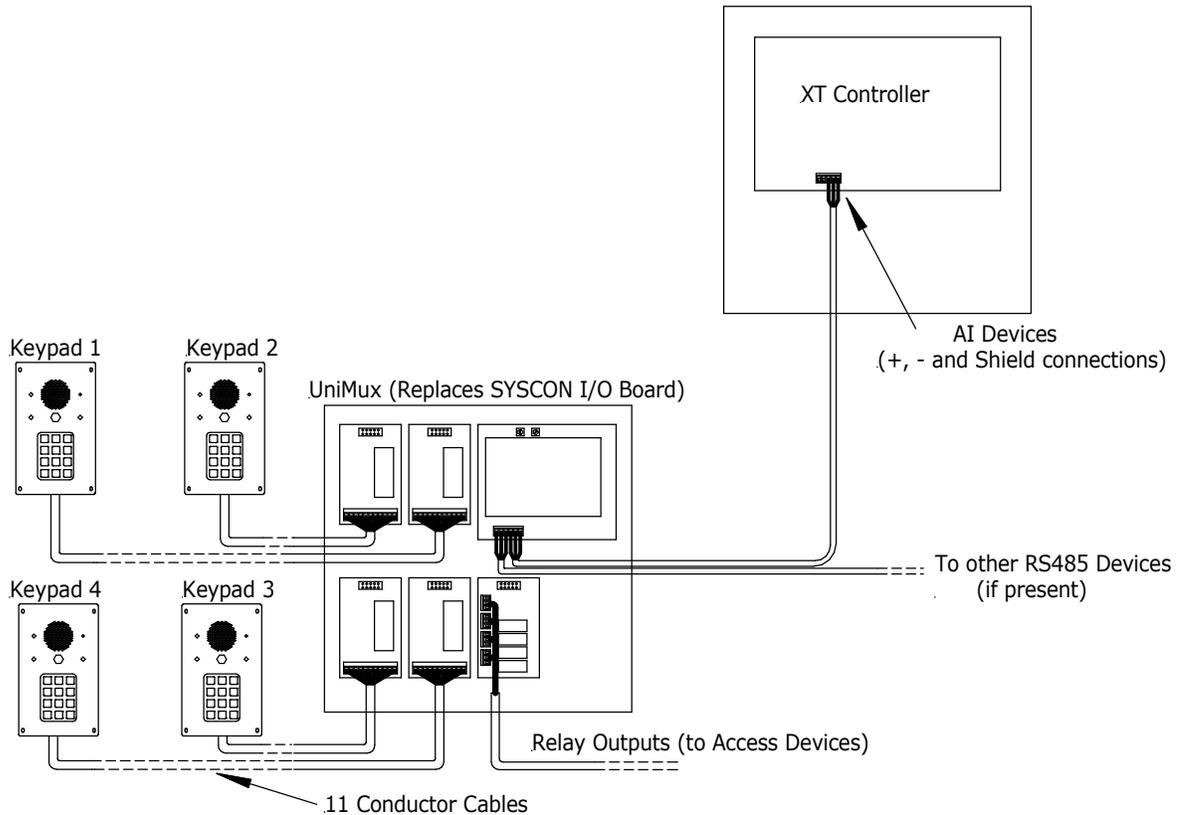
Refer to Chapter Six in the document “1100-044 DigiGate 700 System Installation Manual with Uni-MUX” (<http://www.ptisecurity.com/download/digigate-700-system-installation-manual-including-uni-mux/>) for instructions on how to install this UniMux. Connect the keypads that were originally attached to the Syscon to the daughterboards inside the UniMux (Page 6-3 of document 1100-044). Keypad #1 connects to the terminals on Daughterboard A, Keypad #2 on daughterboard B, and so on.
