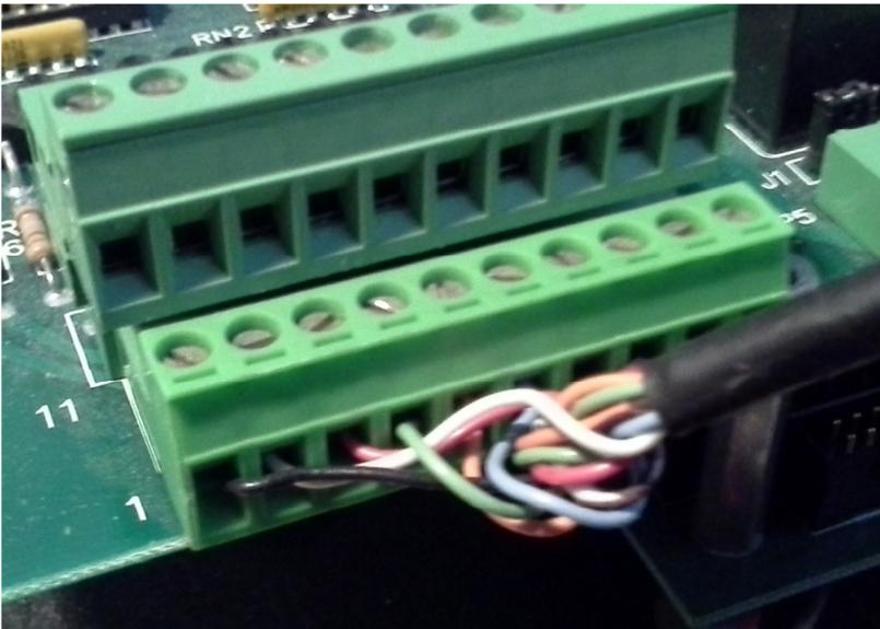
2. Disconnect and label any relay outputs from the keypad interface board.
