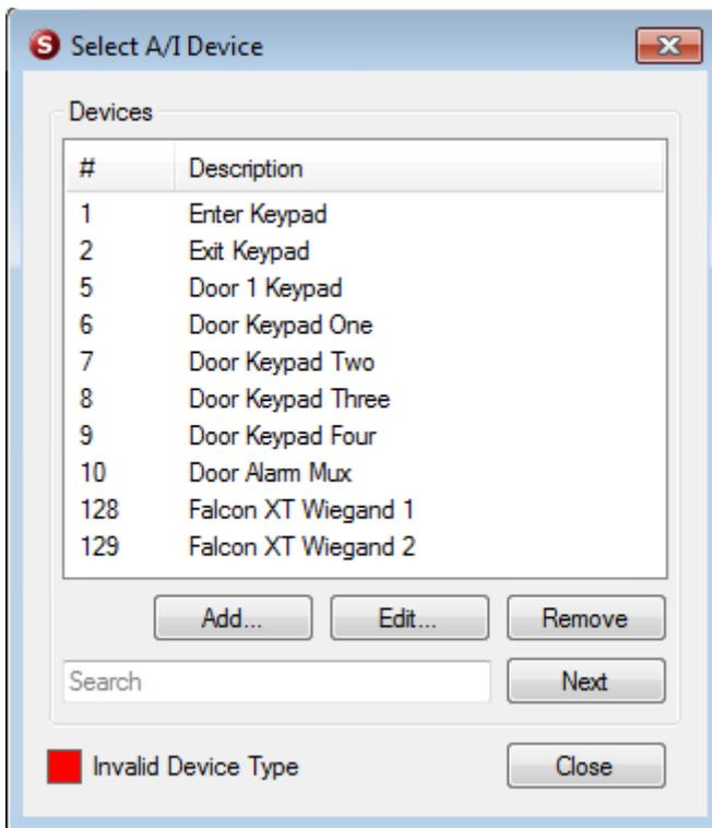
**Note:** Even though the list of Devices shows “Falcon XT Wiegand 1” and “Falcon XT Wiegand 2”, the built-in Wiegand ports of the XT **do not function** when the system is in Digi mode.
