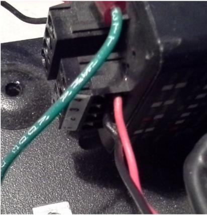
4. Disconnect and label any siren or alarm system trigger wires connected to port P3 on Syscon bottom board, if any are connected.
