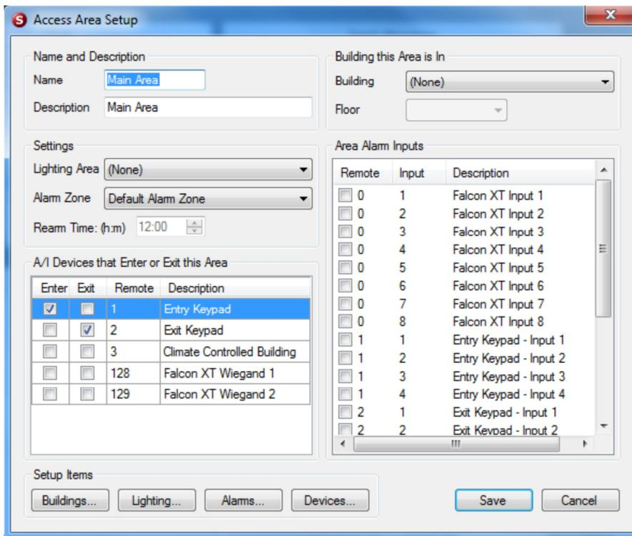
You can see that the Enter Keypad is selected to “Enter” the area, and the exit keypad to “Exit”. For our example site, a second Access Area would be added to the setups, that has the Climate Controlled Building keypad set to “Enter” the area.
