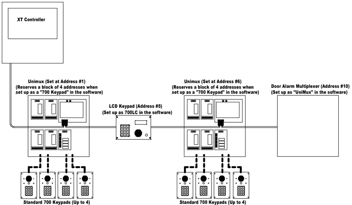
The example on the previous page shows a Keypad UniMux that replaced the Syscon, and is set to address #1. The addresses from 1 through 4 are reserved in the programming setups for standard keypads (i.e. all 4 addresses are reserved even if less than 4 keypads are actually connected to the UniMux).
