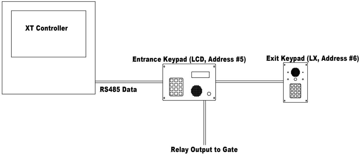
The next example shows a system that had a Keypad Expansion MUX at address #6, to plug in a standard keypad being used for in-car elevator control. Also, the system had 3 Door Alarm Muxes addressed as devices 7, 8 and 9. Because the expansion MUX is an older style and does not have a changeable address (see picture on next page), it was replaced with a UniMux and its address moved to #10. In the setups, all items that were assigned to board #6 are changed to board #10.
