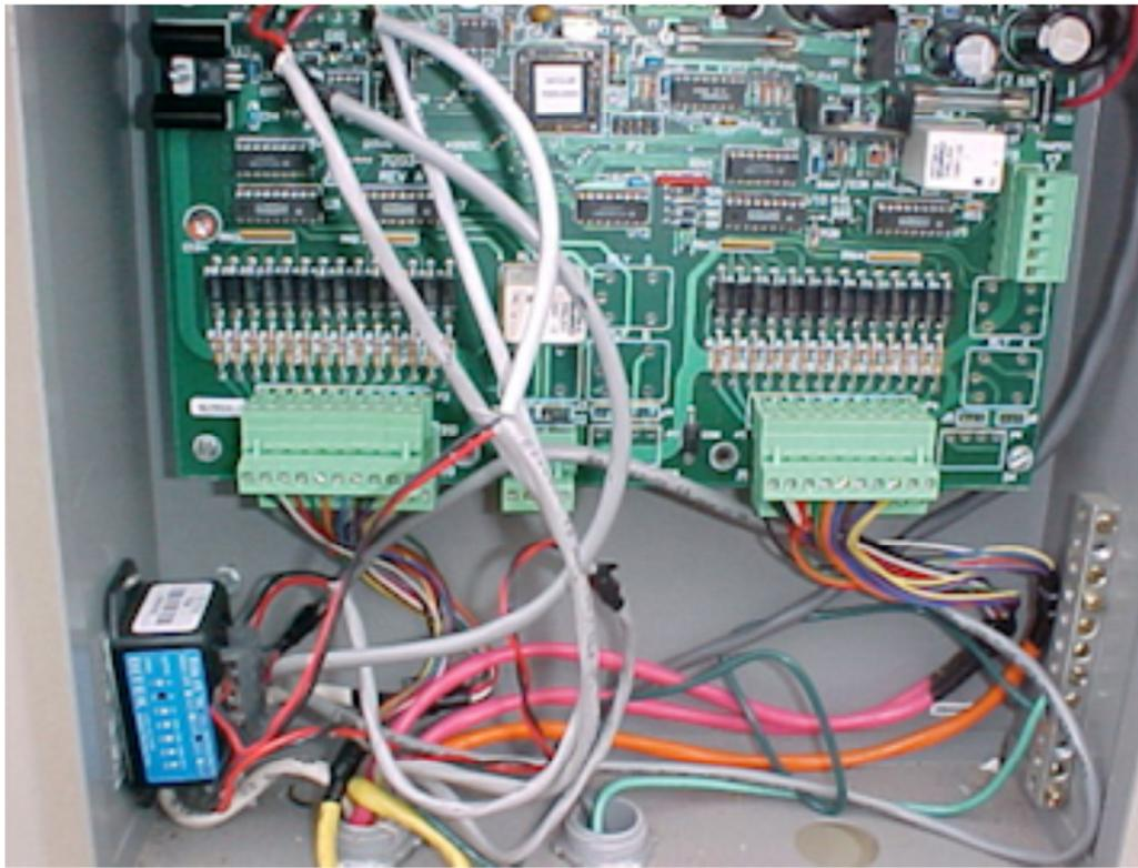
Note at the top of the board there is a square chip with a label. This label has the RS485 address of the mux listed on it, and this address is permanently programmed into that chip and cannot be changed. The chips are no longer available.
