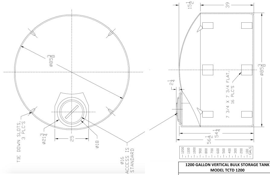
ALL DIMENSIONS SHOWN ARE OUTSIDE PART DIMENSIONS IN INCHES, AND VARY BY THE STANDARD ROTATIONAL MOLDING TOLERANCE OF ±2%.
