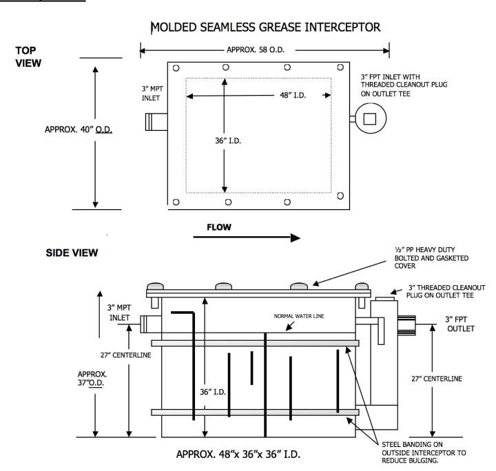
**NOTE:** SEPARATE 3" FLOW CONTROL TEE FURNISHED WITH RESTRICTOR PLATE 3" CONNECTIONS ARE STANDARD ON THIS UNIT. (4" CONNECTIONS ARE AVAILABLE, ONLY IF NEEDED.)
