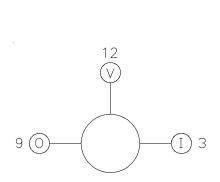
Inlet (I), Outlet (O) and Vent (V)
