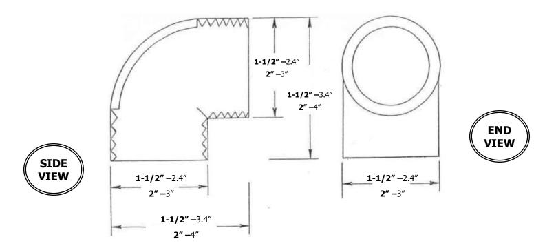
1-1/2" **AND** 2" THREADED <u>POLYPROPYLENE</u>, 90-DEGREE ELBOW, SHORT RADIUS.
