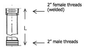
Practical sink strainer adapters', with an extra long tailpiece assembly; the plain-end pipe tailpieces can be readily cut, at the bottom, to accommodate varying rough-in dimensions.
