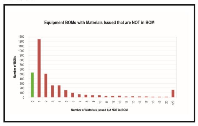
The completeness and accuracy of the equipment BOMs were analyzed as the client was not meeting SIAs in support of maintenance execution. The cost associated with re-active work orders is generally accepted as six times more expensive than preventative maintenance.
