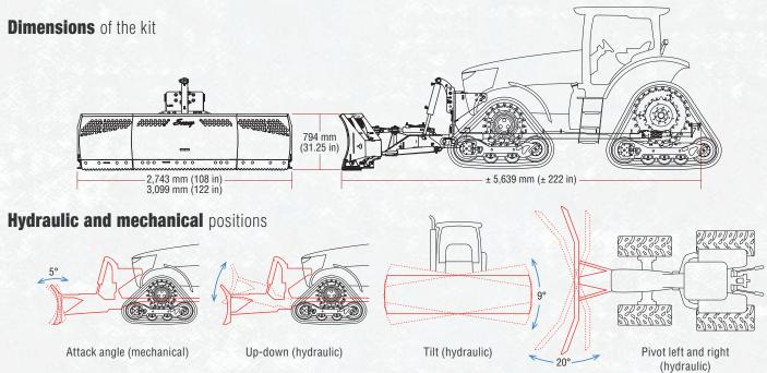
**Features:** 6-way hydraulic positions with adjustable speed action and 2-way mechanical positions to level or push snow. **Kit weight:** ± 953 kg (± 2,100 lbs)
