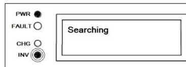
**Searching:** This mode means that the inverter is on and searching for a load. As soon as a load is powered on, it will supply the necessary output voltage.
